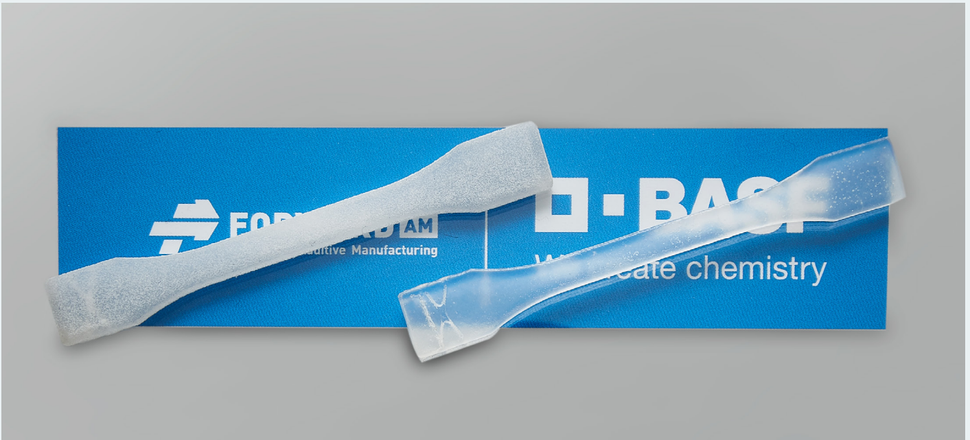
Figure 1: The vapour smoothed test specimen of Ultrasint® PP nat01 (Source: Forward AM).
